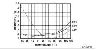
Figure 19. SA605 Application Board, –3dB Limiting (Drop in Audio)
