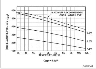
Figure 9. SA605 Application Oscillator Level
