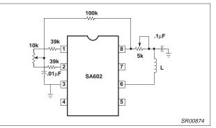
Figure 35. Minimizing RF and LO Feedthrough
