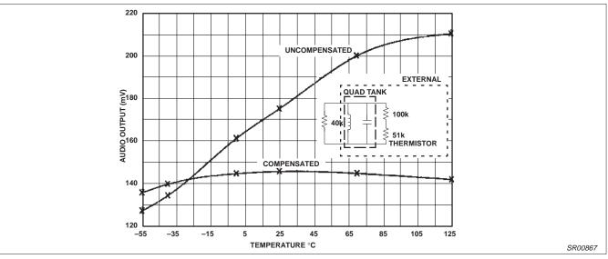
Figure 28. Audio Output: Compensated vs Uncompensated
