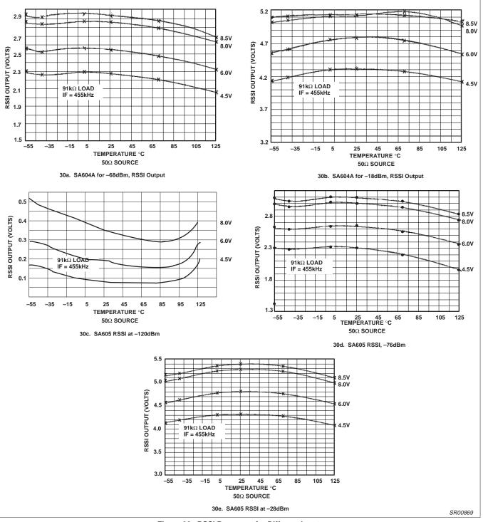
Figure 30. RSSI Response for Different Inputs
