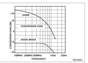
Figure 16. SA605 Conversion Gain vs. Diode Mixer
