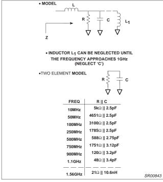
Figure 4. Equivalent Model of RF Input Impedance
