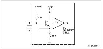
Figure 7. On-board NPN Transistor for Local Oscillator
