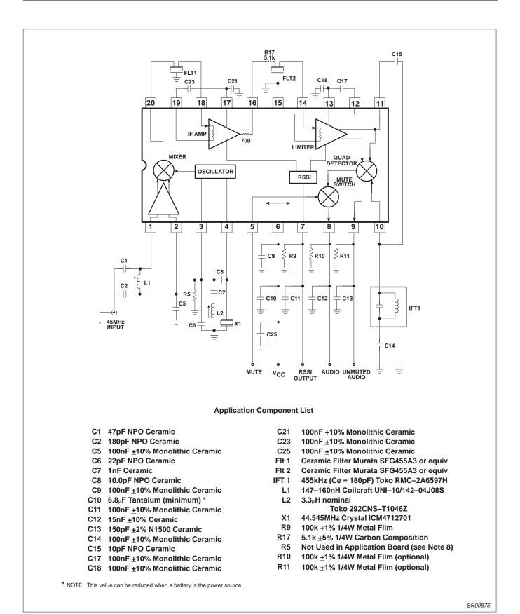
Figure 36. SA605 45MHz Application Circuit
