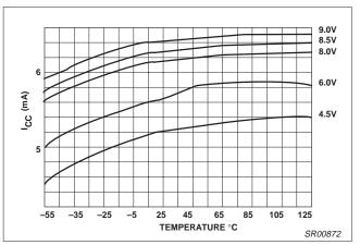
Figure 33. SA605  $I_{CC}$  vs Temperature
