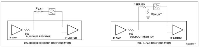
Figure 22. Implementing the 12dB Insertion Loss
