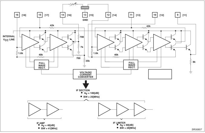
Figure 18. IF Section of SA604A [SA605]
