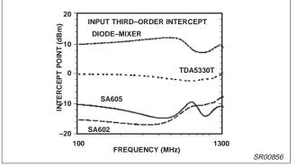
Figure 17. Comparing Different Types of Mixers
