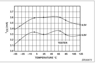
Figure 34. SA604A I<sub>CC</sub> vs Temperature
