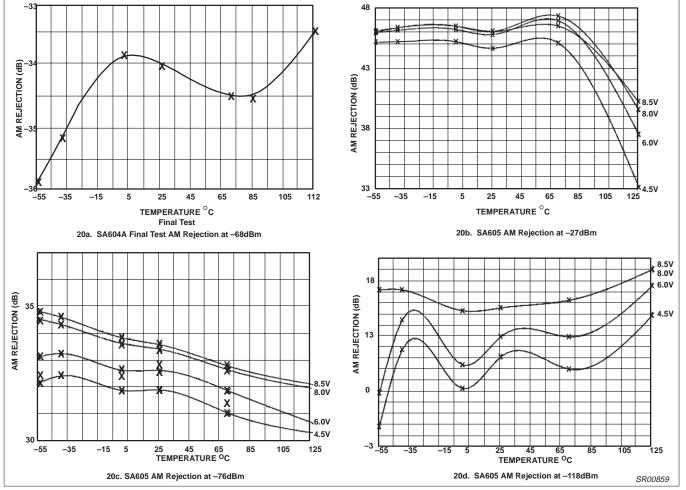
Figure 20. AM Rejection Results at Different Input Levels
