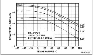
Figure 11. 50 $\Omega$  Conversion Gain
