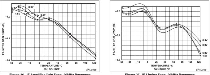
Figure 26. IF Amplifier Gain Drop, 20MHz Response
