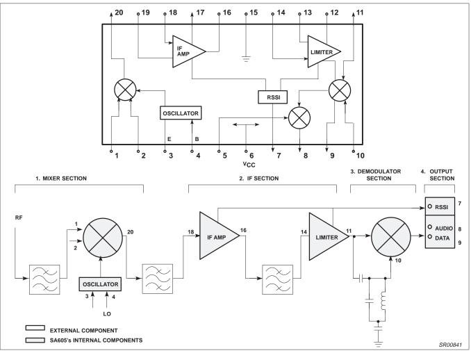
Figure 2. SA605 Broken Down into Four Areas
