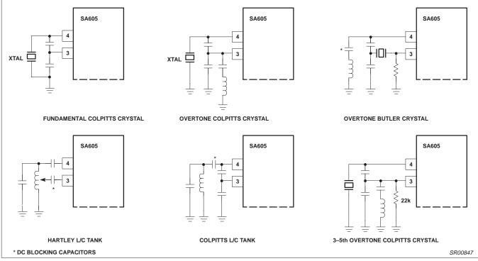
Figure 8. Oscillator Configurations
